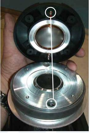
The diaphragm and plate adapter are easily removed from the horn assembly. Notice the terminal locations in relation to the indents of the high frequency driver (circled above).
